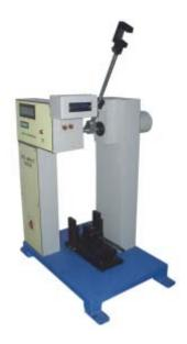
The resistance to breakage by flexural shock of plastics and Electrical insulating materials as indicated by the energy extracted from standardized pendulum type hammers mounted on standardized machines in breaking standard specimens with pendulum swing. The energy absorbed per unit of specimen width is reported in joules.
